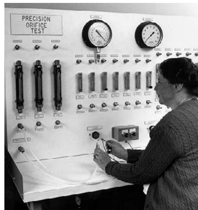
All production orifices are flow tested and must meet exacting flow standards. A special test bench has been constructed for this purpose.
