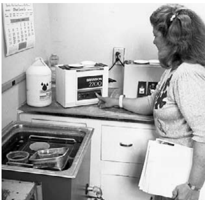
Ultrasonic cleaners are used to remove contamination from the interior of orifice assemblies. Small particles can cause major changes in orifice flow rates.
