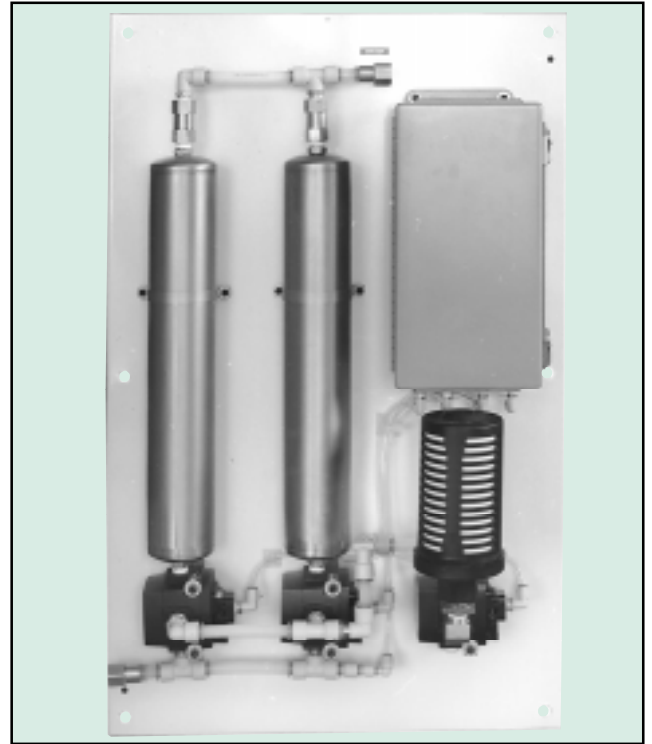
Open frame air dryer module can handle up to 20 scfm at 80 psig and deliver an output dew point of -50°F atmospheric.
